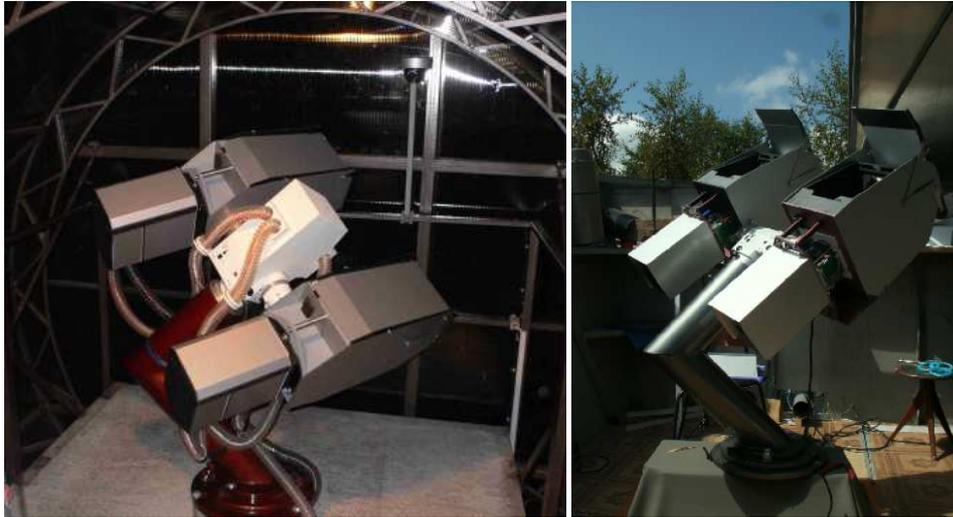
**Fig. 2.** Photos of two channels of MMT installed on a single mount. The complete system consists of 5 such mounts, carrying 9 operative channels and one replacement one.
