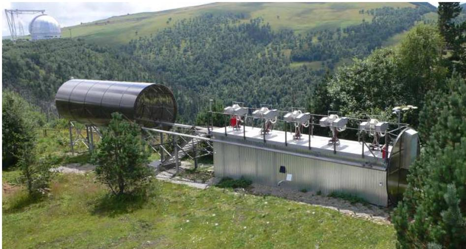
**Fig. 3.** Photo of the all 9 channels of MMT installed on 5 mounts in the single cylindrical dome, which is open at that moment. Russian 6-m telescope may be seen in the background.
